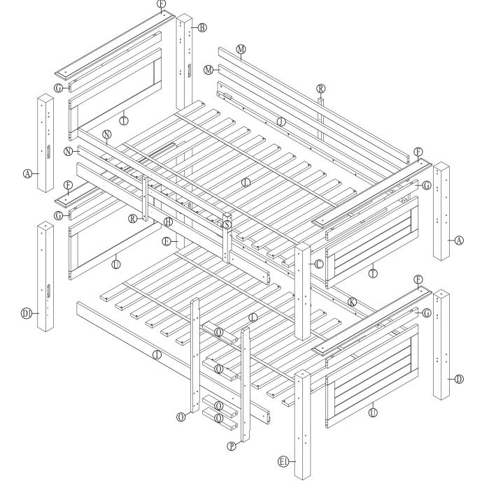
Insert wood dowels (7) into the holes of the headboard top cap (F). Attach headboard top crossbar (G) to headboard top cap (F) with flat head screws (13) as shown. Use a Phillips screwdriver (not included) to tighte flat head screws (13) as shown
