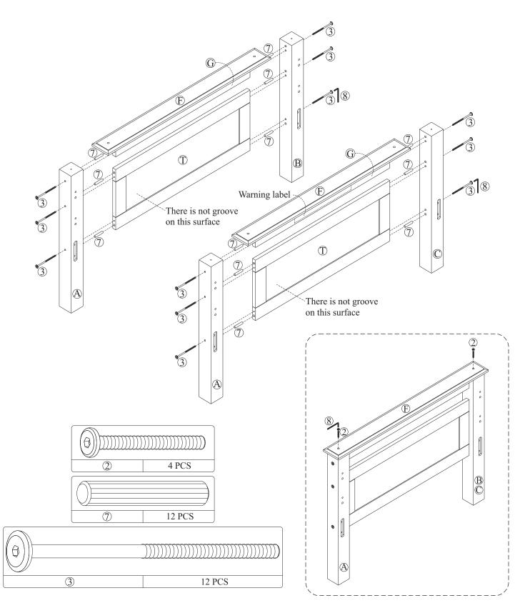
Insert wood dowels (7) into the end holes of headboard top crossbar (G) and lower headboard panel (U). Attach lower post (D1) and (E) to headboard top crossbar (G) and lower headboard panel (U) using bolts (3) as shown. Tighten the bolts (3) with the allen key (8).
