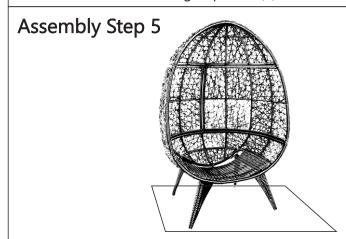
Check for stability and then tighten all Bolts at all joints.
