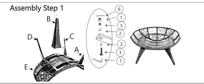
Open the carton and place all the parts onto a clean surface. Unpack all hardware packages. Place the Bottom Seat Panel (E) with its mounting positions, facing upwards, attach Front Left Leg (A) to Bottom Seat Panel (E) using Short Bolt (3), Ring Washers (2), Nut (5), Cap Nut (1) and tighten using Allen Key (7) and Wrench (6). Repeat the same process with Front Right Leg(B), Back Left Leg (C) and Back Right Leg(D). Do not fully tighten the Bolts.
