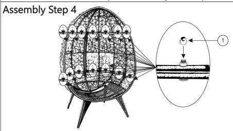
Cover all the Bolts using Cap Nuts (1)
