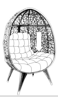
Place the Seat Cushion (I) to the assemled Indah Round Chair w/Feet and once the Seat Cushion is well positioned, secure it by tightening the rope on the back of Seat Cushion (I) to the back frame of Indah Round Chair w/Feet.
