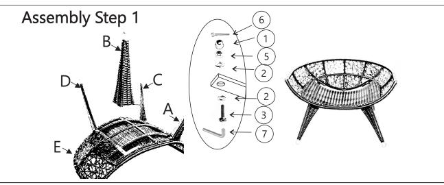
Open the carton and place all the parts onto a clean surface. Unpack all hardware packages. Place the Bottom Seat Panel (E) with its mounting positions, facing upwards, attach Front Left Leg (A) to Bottom Seat Panel (E) using Short Bolt (3), Ring Washers (2), Nut (5), Cap Nut (1) and tighten using Allen Key (7) and Wrench (6). Repeat the same process with Front Right Leg(B), Back Left Leg (C) and Back Right Leg(D). Do not fully tighten the Bolts.
