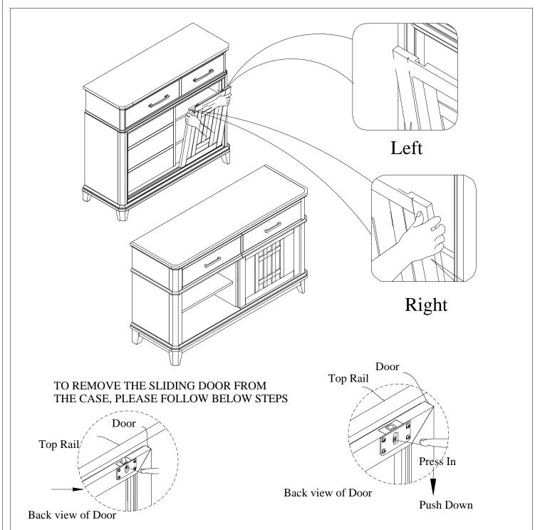
STEP 1: Use your forefingers to press in the buttons at the side of the Latches so that the Latches go up into the U-Track.
