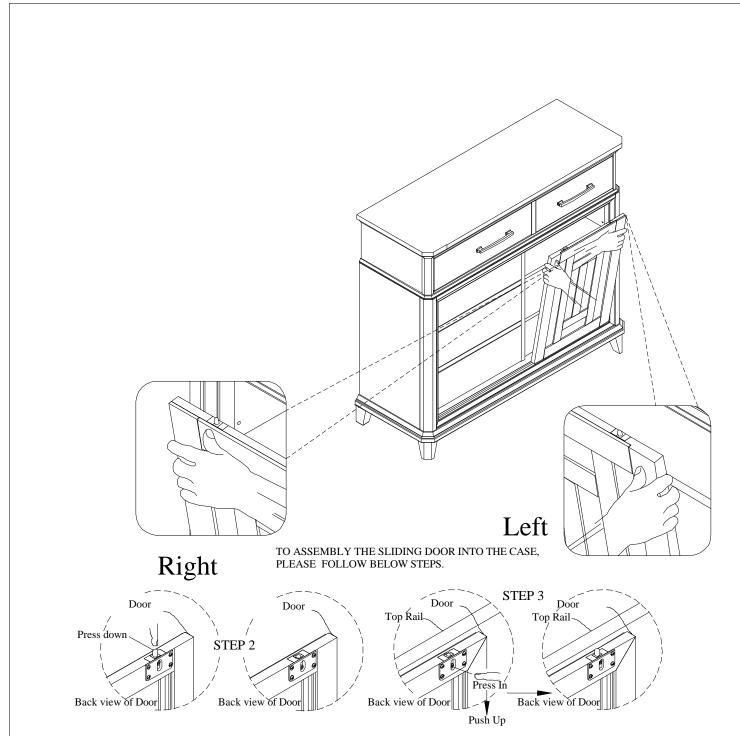
STEP 2: Press down the top latches of door.If the latches are at lower position already, please go to Step3.
