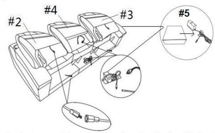
Notes: Follow the direction to connect the power cord as shown from drawing while insert the back rest.
