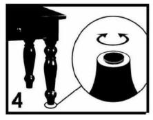
Some furniture comes with height adjustment knobs underneath each leg. To lower or to raise each leg, you need to turn clockwise or counterclockwise, respectively.
