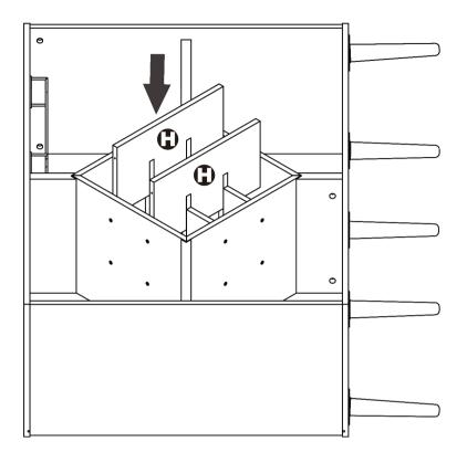
Insert panels (#H) to the other panel (#H) in the unit then secure by using screws (#4).
