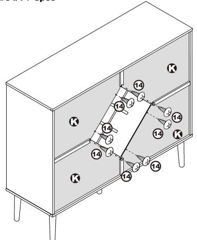
Secure back panels (#K) by using screws (#14).
