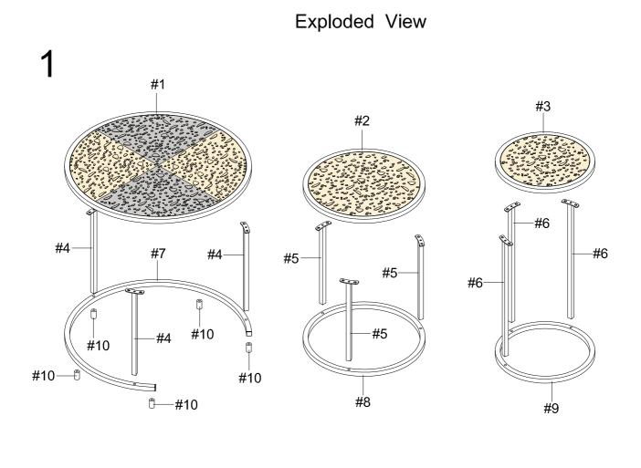
2 #4/#5/#6 Part(#1)x 1pc Align connection tubes (#4,5,6) to #D #A¶ the desktops (#1,2,3) as shown in Part(#2)x 1pc 7 the diagram, then secure by using Part(#3)x 1pc bolts (#A). #1/#2/#3 Part(#4)x 3pcs Part(#5)x 3pcs #6 Part(#6)x 3pcs #4 #5 Hardware(#A)x 18pcs #4 #5 #6 Hardware(#D)x 1pc #6 #5 #1 #4 #2 #3 Į 31
