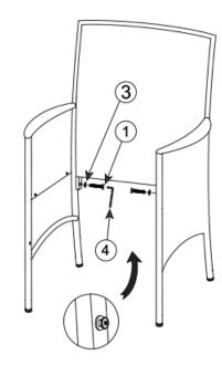
Secure a spring washer (3) and short bolt (1) to each back leg with supplied Allen key (4).
