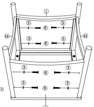
Secure a spring washer (3) and a short bolt (6) with supplied Allen key (7).
