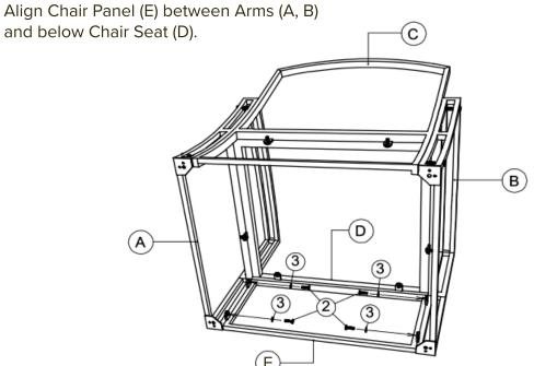
Secure a spring washer (3) and a short bolt (2) with supplied Allen key (7).
