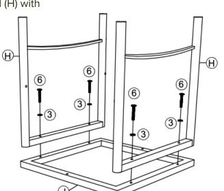
Secure a spring washer (3) and a bolt (6) with supplied Allen key (7).
