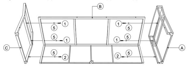
Secure four of the spring washer (5) and bolt (1) with supplied Allen key (8) to seat beams.
