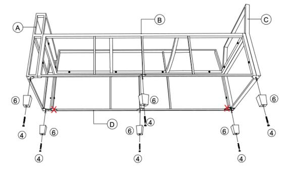
Secure Feet (6) with a long bolt (4) using supplied Allen key (8).
