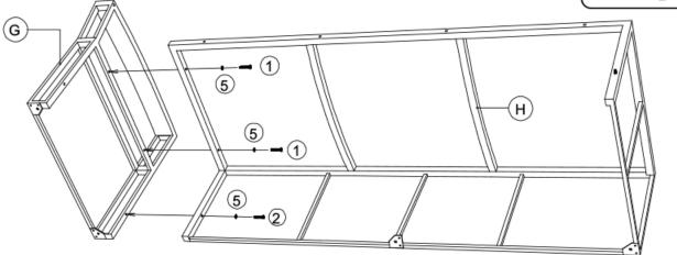
Secure two of the spring washer (5) and bolt (1) with supplied Allen key (8) to seat beams.
