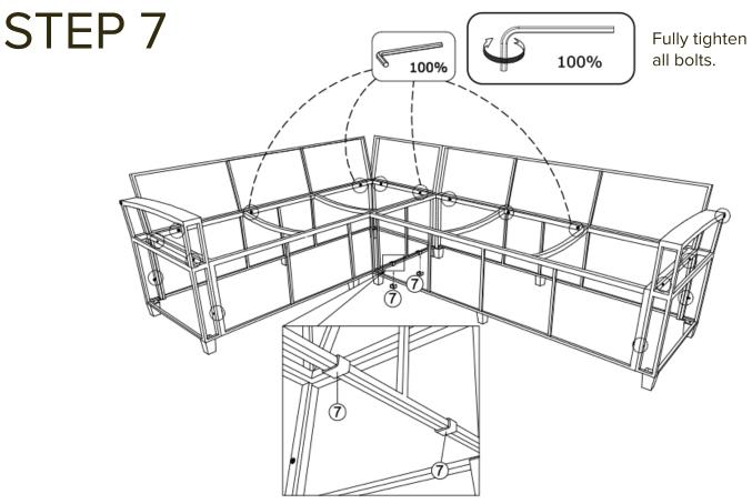
Align Left and Right Benches, then secure with Connection (7).
