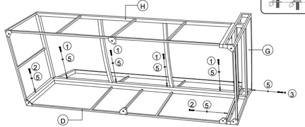
Secure four of the spring washer (5) and bolt (1) with supplied Allen key (8) to seat beam.
