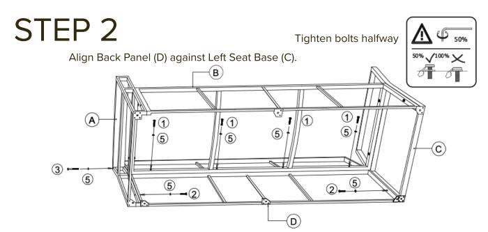
Secure four of the spring washer (5) and bolt (1) with supplied Allen key (8) to seat beams.
