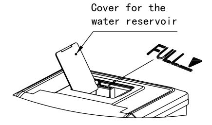
Warning: Do not pour the water into the internal water tank located underneath the ice basket. This tank is not big enough and will effect the ice making performance.
