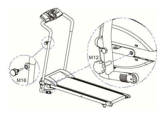
Put M16 stretch know and M12 fix knob to the places as the picture show, then put safety key on the yellow area of panel.
